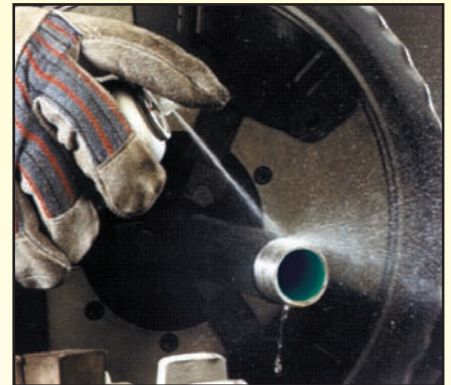
After threading, use a degreasing spray to thoroughly clean the threads and interior of the pipe.
