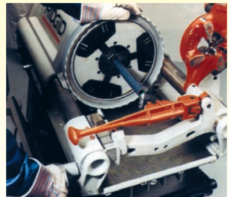
Use a reamer to remove rough edges.
